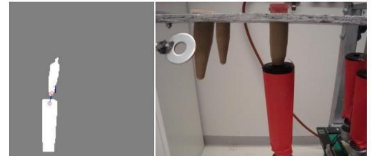
Figure 10. Teat-Cup correspondence for real-time robot visual servoing.
